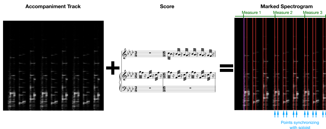
Figure 1: Given a spectrogram of the accompaniment tape and a full score, one can use Info Phil to create a marked track with accompaniment entrances, soloist entrances, and other temporal information.
